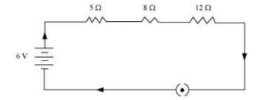
Q2: Redraw the circuit of question 1, putting in an ammeter to measure the current through the resistors and a voltmeter to measure the potential difference across the 12  $\Omega$  resistor. What would be the readings in the ammeter and the voltmeter?
