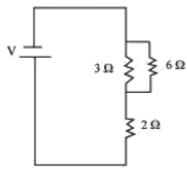
Here, 6  $\Omega$  and 3  $\Omega$  resistors are connected in parallel.
